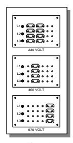
Figure 1 Jumper Link Arrangement
